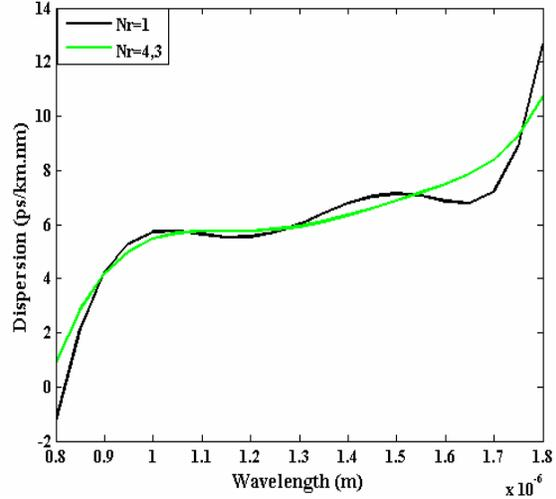
**Fig. 4.** Dispersion curves of F-PCF as a function of wavelength for different number of air hole rings ( $N_r=1, 3$ , and 4) for configuration 1 ( $d_1=5 \mu\text{m}$ ,  $d_2=1.45 \mu\text{m}$ , and  $L=6.75 \mu\text{m}$ ).
