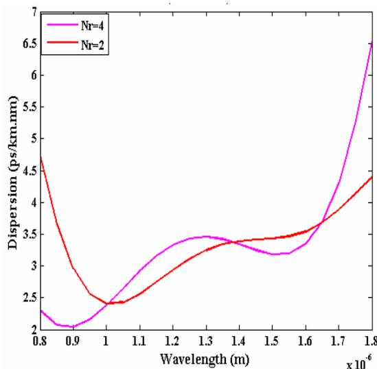
**Fig. 7.** Dispersion curves of F-PCF as a function of wavelength for different number of air hole rings ( $N_r=2$  and  $4$ ) for configuration 3 ( $d_1=5 \mu\text{m}, d_2=1.45 \mu\text{m},$  and  $L=8.75 \mu\text{m}$ ).
