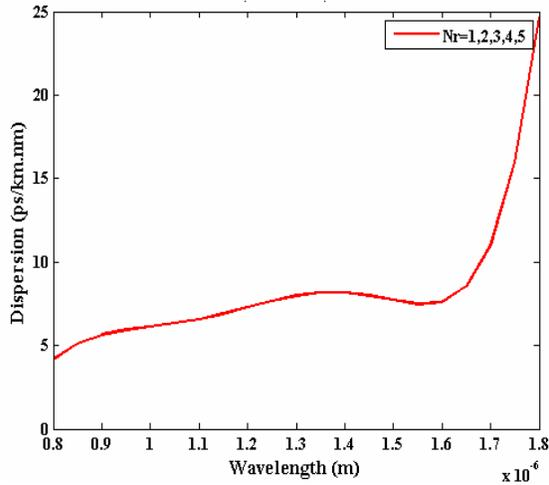
**Fig. 6.** Dispersion curves of F-PCF as a function of wavelength for different number of air hole rings ( $N_r=1, 2, 3, 4,$  and  $5$ ) for configuration 2 ( $d_1=6 \mu\text{m}, d_2=1.75 \mu\text{m},$  and  $L=6.75 \mu\text{m}$ ).
