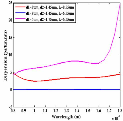
**Fig. 8.** Dispersion curves of F-PCF as a function of wavelength for  $N_r=5$  in different configurations.
