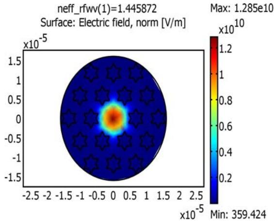
**Fig. 1.** The cross section of the proposed F-PCF with electric field distribution.
