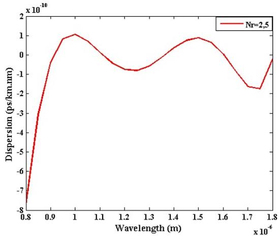
**Fig. 5.** Dispersion curves of F-PCF as a function of wavelength for different number of air hole rings ( $N_r=2$  and 5) for configuration 1 ( $d_1=5 \mu\text{m}$ ,  $d_2=1.45 \mu\text{m}$ , and  $L=6.75 \mu\text{m}$ ).
