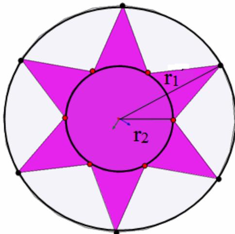
**Fig. 2.** The structure of air holes in more detail,  $d_1=2r_1$  and  $d_2=2r_2$ .
