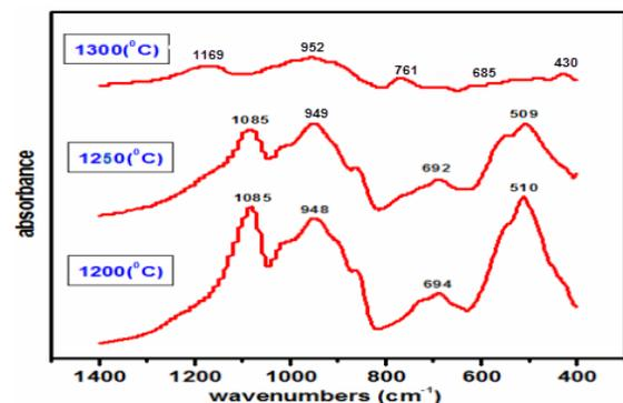
Fig.5: FTIR spectra at 1200°C (bottom spectrum), 1250°C and 1300°C (top spectrum).
