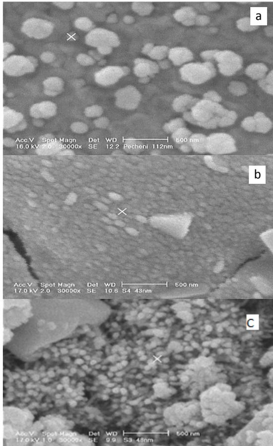
Fig. 3. SEM images of the synthesized  $\alpha$ -cordierite nanocrystallites at different calcinations temperatures: a) 1200°C, b) 1250°C, c) 1300°C.
