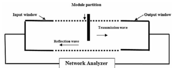
Fig. 4. The experimental setup used to measure dielectric coefficient
