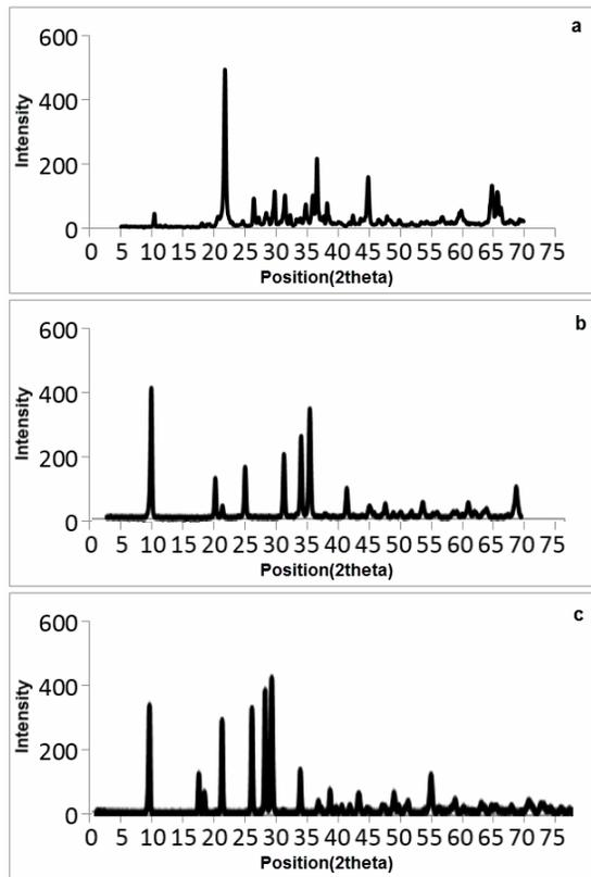
Fig. 1. X-ray powder diffraction patterns of  $\alpha$ -cordierite nanocrystallites calcinated at: a) 1200°C, b) 1250°C, and c) 1300°C.
