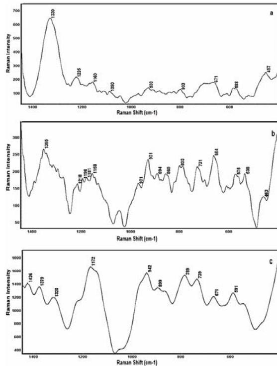
Fig. 2. Raman spectra of the synthesized  $\alpha$ -cordierite nanocrystallites calcinated at: a) 1200°C b) 1250°C c) 1300°C in the spectral region of 200-1500  $\text{cm}^{-1}$ .
