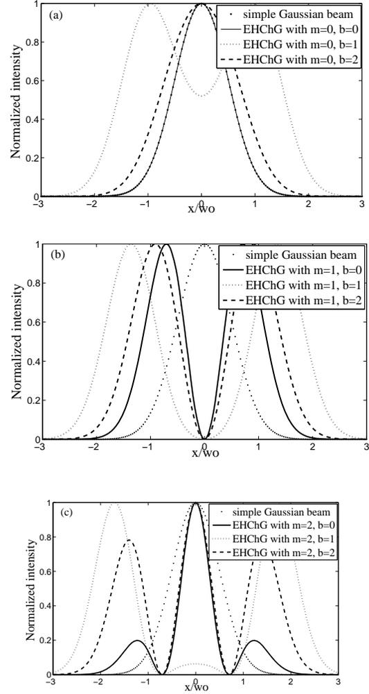
Fig. 2 Electric field distributions of EHChG laser beams at the initial plane, normalized to unity at  $x' = 0$  for various decentered parameters  $b = 1, 2, 3$ . The mode indexes  $m = 0, 1, 2$  are shown in (a), (b) and (c), respectively.
