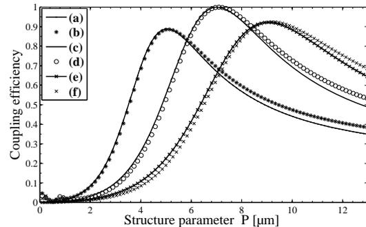
Fig. 3 Comparison of numerical and analytical results. (a) Analytical result for  $L=8.19\mu m$ . (b) Numerical result for  $L=8.19\mu m$ . (c) Analytical result for  $L=12.1875\mu m$ . (d) Numerical result for  $L=12.1875\mu m$ . (e) analytical result for  $L=16.19\mu m$ . (f) numerical result for  $L=16.19\mu m$ .
