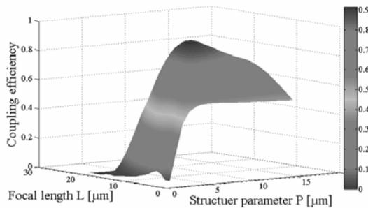
Fig. 5 Coupling efficiency for EHChG laser beam of  $m = 0$  and  $b = 2$  versus structure ( $P$ ) and focal length ( $L$ )
