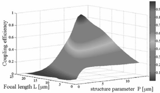
Fig. 4 Coupling efficiency for EHChG laser beam of  $m = 0$  and  $b = 0$  versus structure ( $P$ ) and focal length ( $L$ ).
