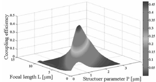
Fig. 6 Coupling efficiency for EHChG laser beam of  $m = 2$  and  $b = 0$  versus structure ( $P$ ) and focal length ( $L$ )
