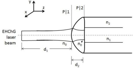
Fig. 1 Schematic diagram of coupling an EHChG laser beam to a single-mode fiber via a quadric lens.
