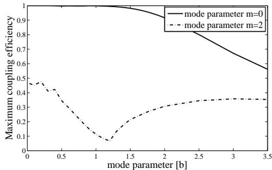
Fig. 7 Maximum coupling efficiency for EHChG laser beam of  $m = 0, 2$  versus mode parameter  $b$ .
