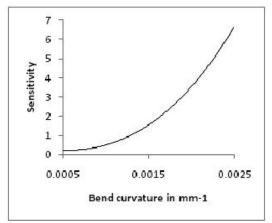
Fig. 5 Improvement in sensitivity with bending curvature
