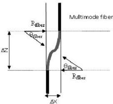
Fig. 2 Structure of the fiber bend.
