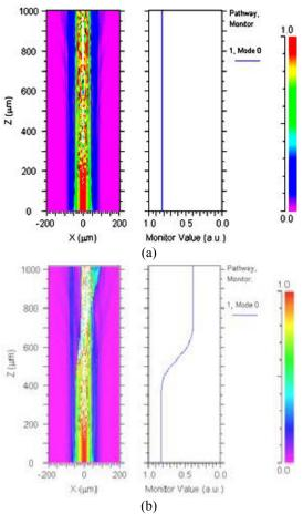
**Fig. 3** Contour map using beam propagation method for (a) straight fiber and (b) bent fiber structure at bend radius of  $R_{\text{fiber}}$ = 2000  $\mu$ m for background index=1.44 and length  $\Delta Z$ =20  $\mu$ m.
