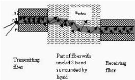
Fig. 1 Basic principle of S bend fiber sensor
