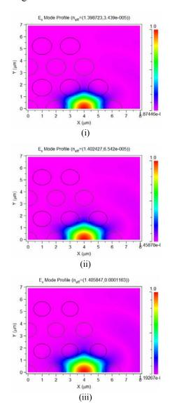
Fig. 2 Simulated Mode Field Pattern of DC-PCF for  $d/\Lambda$  equal to (i) 0.70, (ii) 0.65, and (iii) 0.60 Effective Refractive Index
