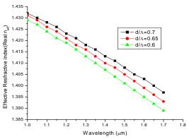
Fig. 3 Variations of effective refractive index spectra for three structures with different  $d/\Lambda$ .
