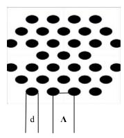
**Fig. 1** Cross section of the proposed DC-PCF (Black and white regions represent air holes and silica, respectively). The structure has three dimensions of d/A of (i) 0.70, (ii) 0.65, and (iii) 0.60
