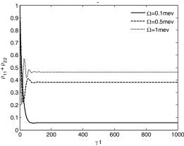
**Fig. 3** Evolution of the upper levels population as a function of normalized time  $\gamma t$  for three different values of  $\Omega$ . Other parameters are  $\gamma_{10}=0.554meV$ ,  $\gamma_{20}=0.001meV$ ,  $T_e=0$ ,  $\Gamma_{10}=0.554meV$ ,  $\Gamma_{20}=0.005meV$ ,  $\delta=0$ ,  $\Gamma_{12}=2meV$ , and  $\omega_{12}=0.2meV$
