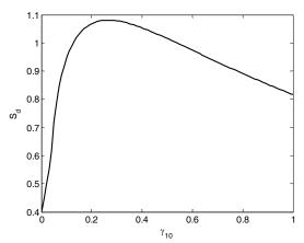
**Fig. 6** Quantum entropy versus intensity of spontaneous emission field for the parameters  $\delta=0.1meV$ ,  $\gamma_{20}=0.1meV$ ,  $\Gamma_{12}=2meV$ ,  $\Gamma_{10}=0.554meV$ ,  $\Gamma_{20}=0.005meV$ ,  $T_{e}=0.5meV$ , and  $\omega_{12}=0.2meV$ .
