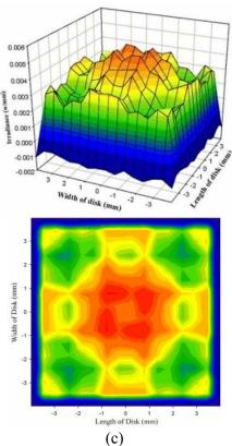
**Fig 4.** Absorbed pump light distribution profiles with their contour profiles of different Yb<sup>+3</sup> ions concentration, a) 12% Yb<sup>+3</sup> atom, b) 14% Yb<sup>+3</sup> atom and c) 20% Yb<sup>+3</sup> atom, respectively.
