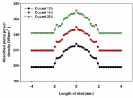
**Fig 5.** 2D comparison of absorbed pump light distribution through the disk for 12, 14 and 20 % of  $Yb^{3+}$  ions concentration, respectively.
