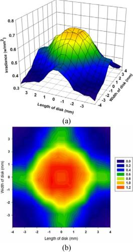
**Fig 2.** a) Irradiance distribution of the pump light profile through the disk, b) Contour profile of pump light irradiance which is indicated the homogeneity of pump light distribution in the center of the disk
