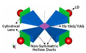
**Fig. 1:** Schematic view of Yb:YAG disk laser with four non-symmetric hollow ducts of side-pumped configuration.
