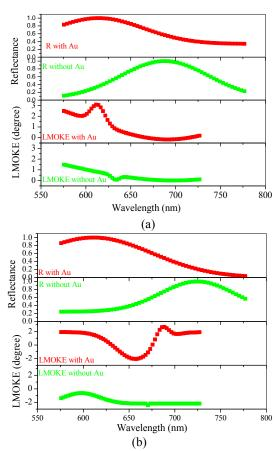
**Fig. 3:** Optical and magneto-optical response of Ce:YIG thin films with Au nanoparticles as compared with single Ce:YIG thin film on the (a) Quartz substrate and (b) Si substrate.
