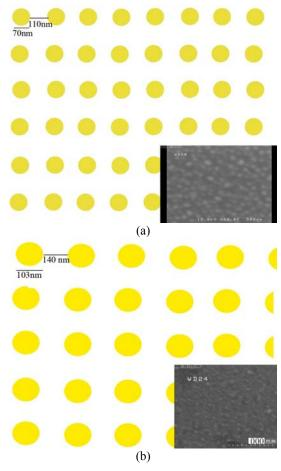
**Fig. 2:** FE-SEM image of Ce:YIG thin films with Au nanoparticles on the (a) Quartz substrate and (b) Si substrate.
