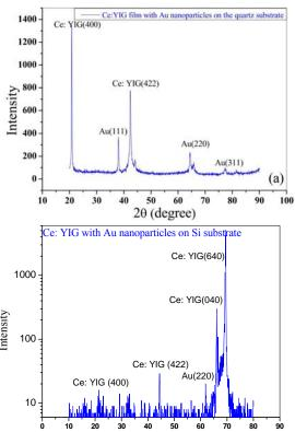
**Fig. 1:** XRD of Ce:YIG thin films with Au nanoparticles on the (a) Quartz substrate and (b) Si substrate.
