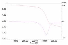
Fig. 3: TG plot of MEH-PPV.
