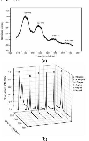
**Fig. 5:** (a) Emission spectrum of MEH-PPV solution at lower concentration and (b) Dual ASE at higher concentrations of MEH-PPV solution. Relative intensities of two peaks are varied with concentration.
