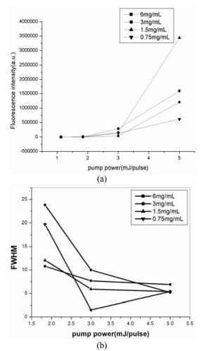
**Fig. 7:** (a) Fluorescence intensity of MEH-PPV and (b) FWHM of ASE vs. pump power for different concentrations
