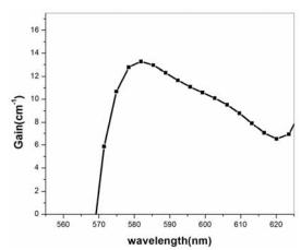
Fig. 8: Gain spectrum of MEH-PPV solutions
