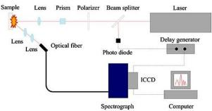
Fig. 2. Scheme for LIBs setup
