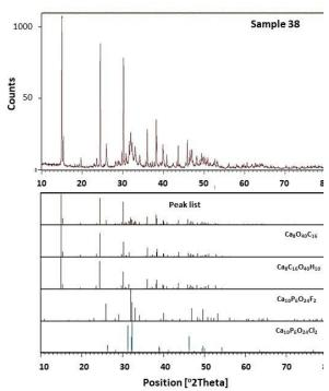
Fig. 5 XRD results identifying the crystalline components of Sample 38, mainly Whewellite and Fluorapatite
