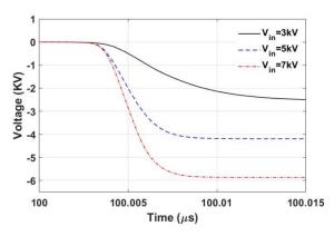
Fig. 5. Rise time of the generated pulses in Fig. 2.
