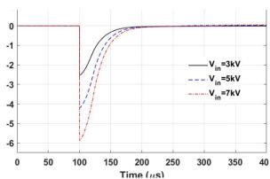
Fig. 2. Generated pulses at supply voltages of 3, 5, and 7kV.
