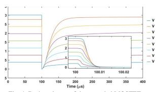
Fig. 4. Drain voltages of the cascaded MOSFETs at the moment of switching, illustrating the sequential turn-on behavior and the stepwise voltage drop across the series.
