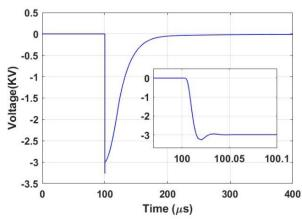
Fig. 7. Damping of the resonance generated at the pulse edge by series connection of appropriately selected resistors at the circuit output.
