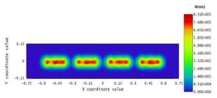
Fig. 1. Intensity pattern of laser bars at a distance of 1.1 mm from diode laser
