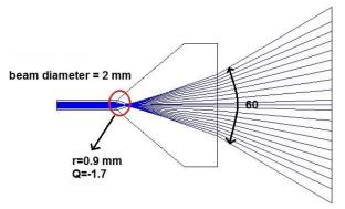
Fig. 4. Powell lens geometry for laser line generation.
