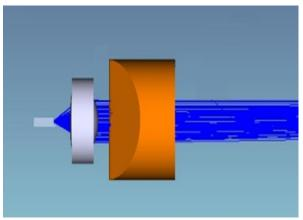
Fig. 5. Arrangement of laser diode, collimating lens and Powel lens in ZEMAX software
