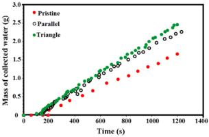
Fig. 7. Mass of collected water versus time for pristine and surface patterned brass sheets.
