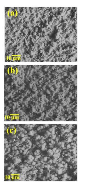
Fig. 4. SEM images of irradiated brass surfaces: (a) B1, (b) B2, and (C) B3.
