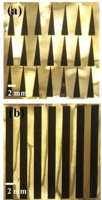
Fig. 2. The optical images of fabricated (a) triangular and (b) line parallel patterns on brass foil.
