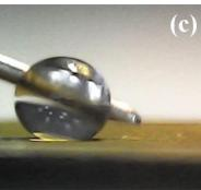
Fig .6. Indicating the SHB behavior of the irradiated brass surface (B1) after 60 days.
