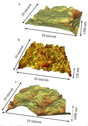
Fig. 5. AFM images of (a) non-irradiated and irradiated samples at fluence of 5 J/cm² and at a repetition rate of 10 Hz with scanning velocity of 64  $\mu$ m/s in X-direction and Y-displacement of (b) 100, and (c) 250  $\mu$ m.
