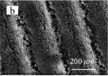
Fig. 3. (a) microscopic and (b) FESEM image of the sample irradiated at the fluence of 5 J/cm $^2$ , with scanning velocity of 64  $\mu$ m/s in X-direction and Y-displacement of 250  $\mu$ m.
