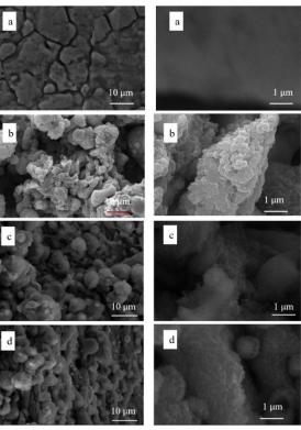
Fig. 4. FESEM images of (a) non-irradiated and irradiated samples at fluence of 5 J/cm<sup>2</sup> and at a repetition rate of 10 Hz with scanning velocity of 64  $\mu$ m/s in X-direction and Y-displacement of (b) 250 (no overlapping in Y-direction), (c)150 and (d) 100  $\mu$ m with two different magnifications.
