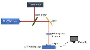
Fig. 2. Schematic diagram of experimental setup. Scanning velocity in X-direction is 64  $\mu$ m/s, while the displacement of two x-lines is adjusted by the working stage.
