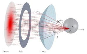
Fig. 3. Focusing of paraxial rays [6].
