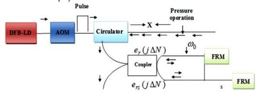
Fig. 1. Schematic illustrates the optical path in a Michelson interferometer, which incorporates a distributed feedback laser diode (DFB-LD), an acoustic-optic modulator (AOM), and a Faraday rotator mirror (FRM) [20].
