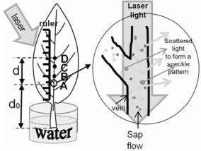
**Fig. 2.** In speckle imaging technique, a dry leaf is irrigated with water and a laser light is irradiated onto the leaf and the scattered light forms a speckle image of the leaf. By analysis of the speckle image, water flow in the leaf can be monitored.
