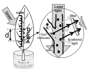
**Fig. 1.** In fluorescent imaging technique, a leaf is irrigated with the solution of water and dye molecules and a laser light is irradiated onto the leaf. By tracing dye molecules, water flow in the leaf can be monitored.
