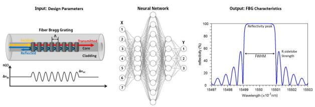
Fig. 1. The plan of the FBG structure and NN architecture for prediction of output parameters. An NN architecture was employed to predict the features of the FBG based on the design parameters.
