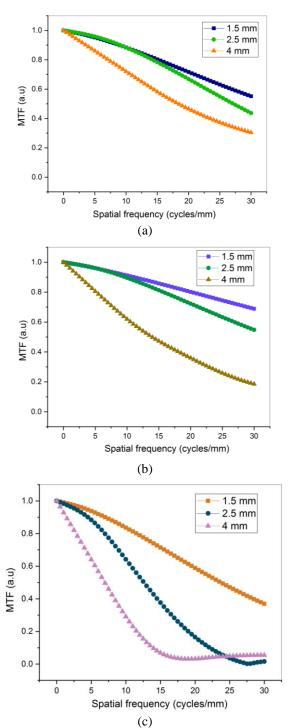
Fig. 1<sup>\gamma</sup>. The MTF comparison between the treated eyes for three pupil diameters in three vision modes: a) far, b) intermediate c) near.
