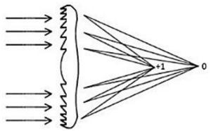
Fig. 4. The structure of a multifocal diffractive lens.
