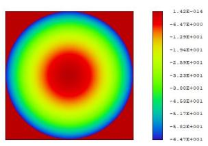
Fig. 7. Surface phase map of the designed multifocal diffraction lens.
