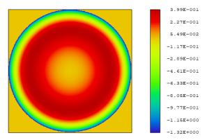
Fig. 6. Sag of the designed diffractive multifocal lens
