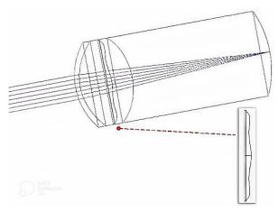
Fig. 5. Layout of designed diffractive IOL.
