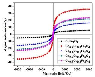
Fig. 5. The diagram of M-H samples.
