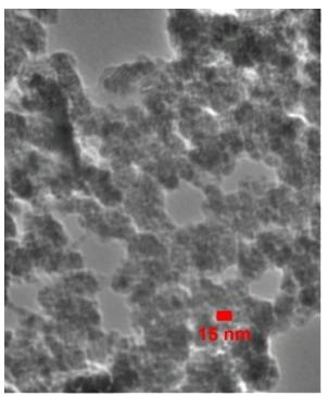
Fig. 4. The TEM images of Co<sub>0.4</sub>Cu<sub>0.6</sub>Fe<sub>2</sub>O<sub>4</sub> sample.
