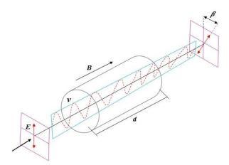
Fig. 1. The schematic scheme of Faraday effect.
