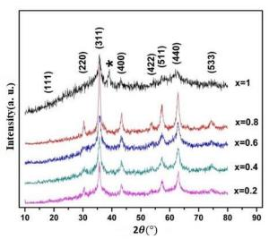
Fig. 2. X-ray diffraction pattern of copper cobalt ferrite samples. For example, there is (x=1) a peak corresponding to the plate (111) of copper oxide according to the reference card 01-080-0076, which is marked with an asterisk (\*).
