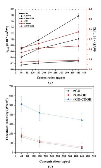
Fig. 5. (a) Nonlinear refractive index & thermoptical coefficient, (b) Threshold intensity.
