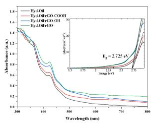
Fig. 2. Absorbance spectrum of hydraulic oil alone and with 440  $\mu$ g/cc concentration of rGO, rGO-OH, and rGO-COOH nanosheets. The inset figure shows the derived Tauc diagram.
