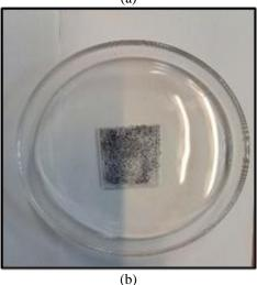
Fig. 1. The image of (a) rhodamine 6G solution and (b) crystal violet solution, deposited on the graphene-based substrate by solution soaking.
