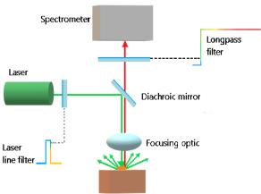
Fig. 3. Schematic diagram of the Raman spectrometer
