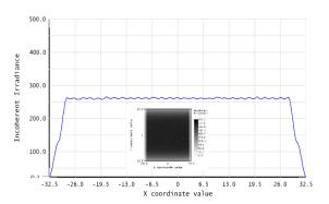
Fig. 3. The pump intensity distribution (W/cm²) vs. slab thickness for design#2 slabs with 5000W optical pumping from each side (inset: the pump distribution in the slab faces).
