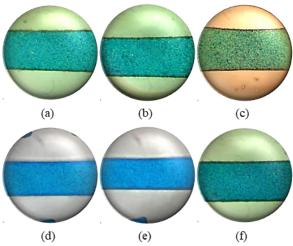
**Fig.** 5. Images of SPE-60 molds with different thicknesses. (a)  $25\mu m$ , (b)  $35\mu m$ , (c)  $45\mu m$ , (d)  $65\mu m$ , (e)  $95\mu m$ , (f)  $130\mu m$ .
