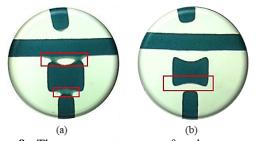
**Fig. 9.** The poor pattern transfer due to weak contact causes light diffraction. (a), (b) Poor transmission of the optical system from the photomask to the film that affects the performance of the mold.
