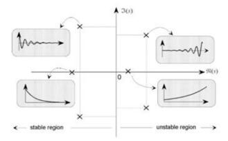
Fig. 7. The type of dynamic behavior of the system according to the positive and negative areas of the real and imaginary parts of the roots [26].
