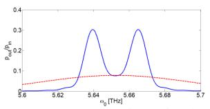
Fig. 7. Output pulse power as a function of a carrier frequency for the duration of input pulse  $\tau_0 = 0.56$  ps (red dashed line) and  $\tau_0 = 5.6$  ps (blue solid line).
