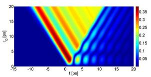
Fig. 8 Time envelope of the output pulse  $\left|E_{\scriptscriptstyle out}\left(t\right)\right|/E_{\scriptscriptstyle 0}$  as a function of the input pulse duration  $\tau_0$  for carrier frequency  $\omega_c$ . The color depicts the value of  $\left|E_{\scriptscriptstyle out}\left(t\right)\right|/E_{\scriptscriptstyle 0}$ .
