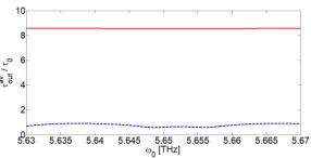
Fig. 6. Average duration of the output pulse as a function of a carrier frequency for the duration of input pulse  $\tau_0 = 0.56$  ps (red solid line) and  $\tau_0 = 5.6$  ps (blue dashed line).
