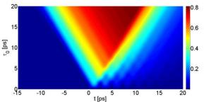
Fig. 9. Time envelope of the output pulse  $|E_{\scriptscriptstyle out}(t)|/E_{\scriptscriptstyle 0}$  as a function of the input pulse duration  $\tau_0$  for carrier frequency  $\omega_l$ . The color depicts the value of  $|E_{\scriptscriptstyle out}(t)|/E_0$ .
