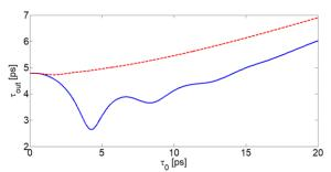
Fig. 10. Duration of output pulse as a function of the input pulse duration  $\tau_0$  for carrier frequency  $\omega_c$  (blue solid line) and  $\omega_l$  (red dashed line).
