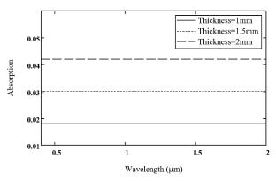
Fig. 8. Total absorption spectra for different layer thickness, which shows constant response. The same is for reflection and transmission. The other simulation parameters are:  $\beta$ =30°,  $\lambda$ =1.3 $\mu$ m,  $\mu$ a=0.1cm<sup>-1</sup>,  $\mu$ s=100cm<sup>-1</sup>, and g=0.9.
