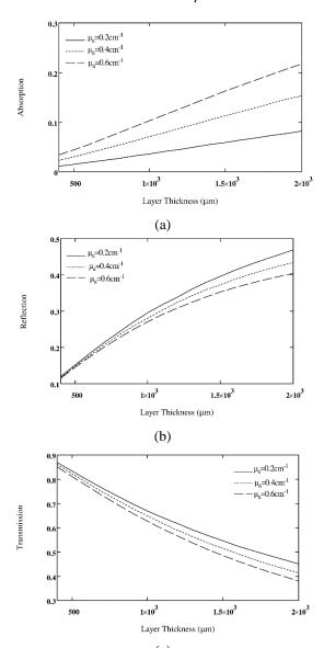
Fig. 7. (a) Total absorption, (b) total reflection and (c) total transmission vs layer thickness and for different  $\mu$ a. We calculate this for different  $\mu$ a=0.2, 0.4, and 0.6 cm<sup>-1</sup>. The other simulation parameters are:  $\beta$ =30°,  $\lambda$ =1.3 $\mu$ m,  $\mu$ s=100cm<sup>-1</sup>, and g=0.9.
