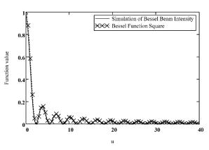
Fig. 2. Verification of Bessel beam. The line curve gives the simulation intensity upon using the appendix accept/rejection technique. The dotted-crosses curve gives the Bessel square as a function of *u*
