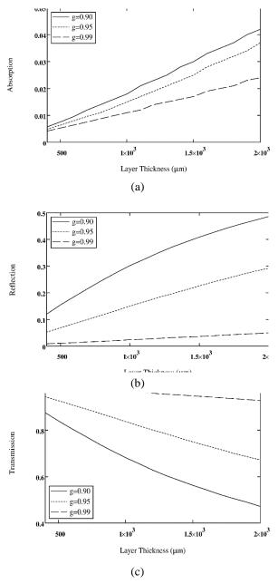
Fig. 5. (a) Total absorption, (b) reflection and (c) transmission as a function of LT for different g. We calculate this for different anisotropy factor g=0.90, 0.95 and 0.99. The other simulation parameters are:  $\beta$ =30°,  $\lambda$ =1.3 $\mu$ m,  $\mu a$ =0.1cm<sup>-1</sup>, and  $\mu s$ =100cm<sup>-1</sup>.
