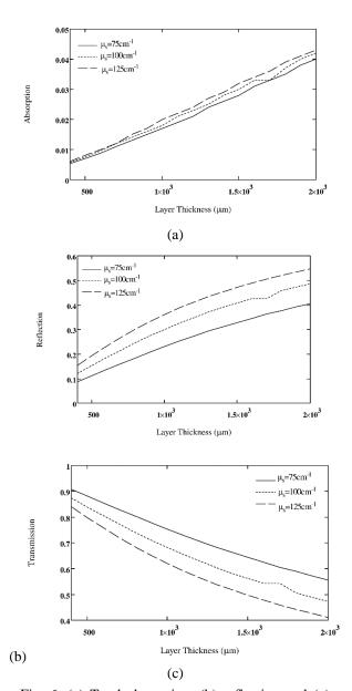
Fig. 6. (a) Total absorption, (b) reflection and (c) transmission vs layer thickness and for different  $\mu s$  of 75, 100, and 125 cm<sup>-1</sup>. The other simulation parameters are:  $\beta$ =30°,  $\lambda$ =1.3 $\mu$ m,  $\mu a$ =0.1cm<sup>-1</sup>, and g=0.9.
