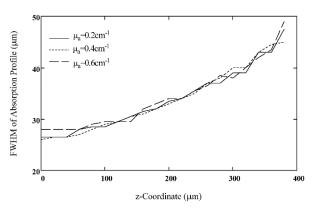
Fig. 10. FWHM for absorption profile along x-direction as a function of depth for different values of  $\mu a$ . The curves show same response of monotonic increasing performance
