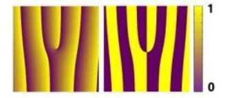
Fig. 2. Fork grating for generation of vortex beam with topological charge l=1. Right: the binary hologram, Left: the blazed hologram.
