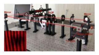
Fig. 6 Mach-Zehnder interferometer setup, the fork grating is obtained from Mach-Zehnder which shows the topological charge one (l=1).
