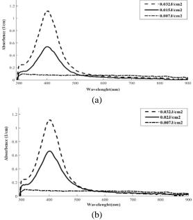
Fig. 4. UV-visible spectrum of Ag NPs at the number of the laser pulses at 1500 and (a) three different laser energy densities:  $0.032 \text{J/cm}^2$  and  $0.015 \text{J/cm}^2$  and  $0.007 \text{J/cm}^2$  (b) three different laser energy densities:  $0.032 \text{J/cm}^2$  and  $0.027 \text{J/cm}^2$  and  $0.007 \text{J/cm}^2$ .
