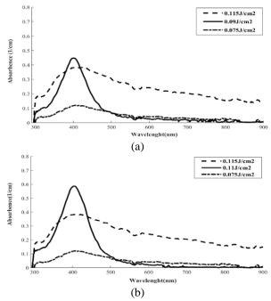
Fig. 3. UV-visible spectrum of Ag NPs at the number of the laser pulses at 900 and (a) three different laser energy densities: 0.115J/cm<sup>2</sup> and 0.09J/cm<sup>2</sup> and 0.075J/cm<sup>2</sup> (b) three different laser energy densities: 0.115J/cm<sup>2</sup> and 0.11J/cm<sup>2</sup> and 0.075J/cm<sup>2</sup>.
