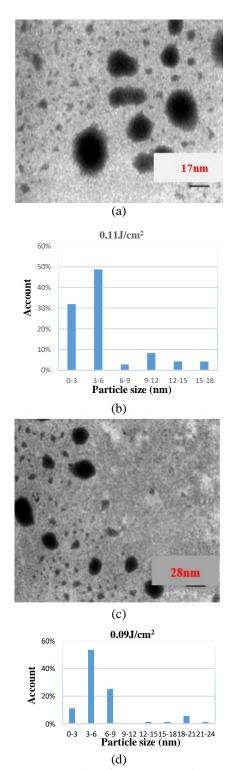
Fig. 5. TEM results of Ag NPs at the optimum number of the laser pulses at 900 at two optimum laser energy densities: (a) 0.11J/cm<sup>2</sup> (Scale Bar=17nm), (b) distribution diagram of Ag NPs for the optimum laser energy density at 0.11J/cm<sup>2</sup> (N=72, mean=5.04nm), (c) 0.09J/cm<sup>2</sup> (Scale Bar=28nm) and (d) distribution diagram of Ag NPs for the optimum laser energy density at 0.09J/cm<sup>2</sup> (N=71, mean=6.34nm).
