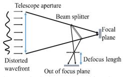
Fig. 8. Getting in-focus and out of focus images.
