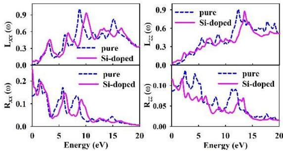
Fig. 5. xx-(left) and zz-components (right) of energy loss (top) and reflectivity (bottom) functions of pure (dashed lines) and silicon-doped (solid lines) Sc2C(OH)2 monolayer.
