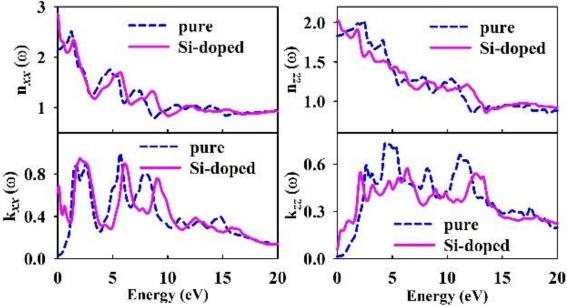
Fig. 6. xx-(left) and zz-components (right) of refraction (top) and extinction (bottom) functions of pure (dashed lines) and silicon-doped (solid lines)  $Sc_2C(OH)_2$  monolayer.
