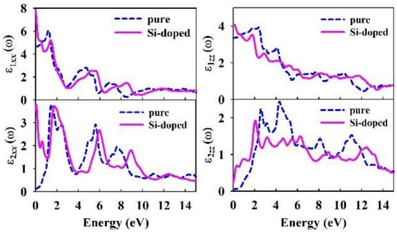
Fig. 4. xx-(left) and zz-components (right) of real (top) and imaginary (bottom) parts of the dielectric functions of pure (dashed lines) and silicon-doped (solid lines)  $Sc_2C(OH)_2$  monolayer.
