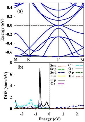
Fig. 3. (a) Band structure and (b) partial DOS of silicon-doped  $Sc_2C(OH)_2$  monolayer. Band inversion occur at the  $\Gamma$  point near the Fermi level.
