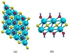
Fig. 1. The top (a) and side (b) views of a  $3\times3$  supercell of  $Sc_2C(OH)_2$  monolayer.
