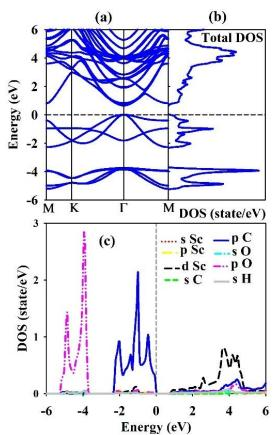
Fig. 2. (a) Band structure, (b) Total DOS, and (c) partial DOS of pure Sc<sub>2</sub>C(OH)<sub>2</sub> monolayer.
