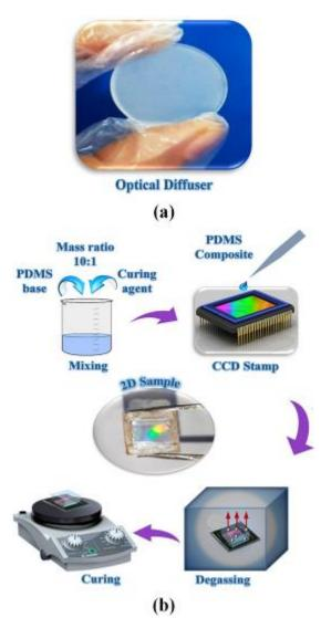
Fig. 1. (a) The real image of the fabricated optical diffuser, and (b) A schematic array of the fabrication process of two-dimensional samples based on PDMS.
