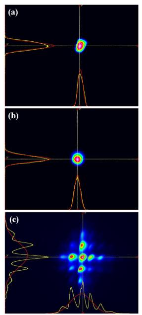
Fig. 3. Recorded images of the spatial intensity distribution for the states: (a) before, (b) after placing the optical diffuser along the optical path, and (c) Spatial intensity distribution of the 2D PDMS-MgF<sub>2</sub> sample by placing the optical diffuser along the optical path. The yellow curves show the measured intensity distribution, and the red curves show the corresponding Gaussian intensity distribution in the x and y directions.
