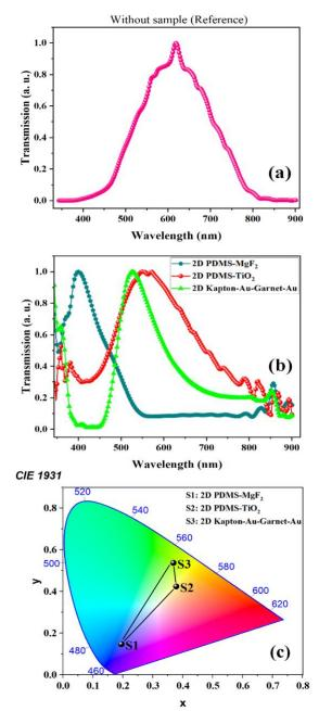
Fig. 4. (a) Measured transmission spectrum of the light source without the presence of the sample, (b) Normalized transmission spectra of the different 2D samples, and (c) The colorimetric diagram of the fabricated 2D samples.
