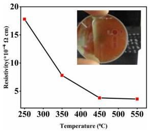
Fig. 5. Sheet resistance vs. annealing temperature  $(250-550 \, ^{\circ}\text{C})$ .
