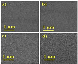
Fig. 3. The SEM images of DBR composed of 5 pairs of SiO<sub>2</sub>/TiO<sub>2</sub>/ITO thin films annealed at a) 250 °C, b) 350 °C, c) 450 °C, d) 550 °C.
