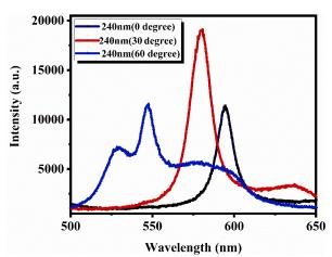
Fig. 8. Electroluminescence spectra of the microcavity OLED with angles of 0, 30 and 60 degrees(on device) detection.
