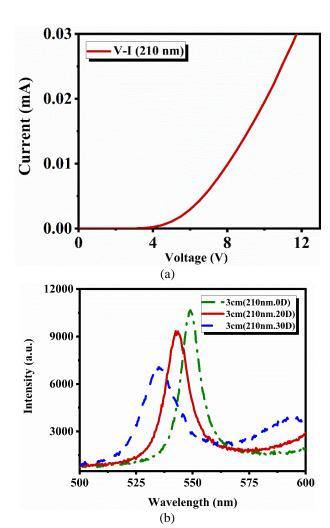
Fig. 9. a) Current density-voltage curves of a 210 nm microcavity and b) EL spectra detection at different angles of 0, 20 and 30 degrees with a 3 cm distance from the device.
