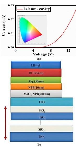
Fig. 7. a) Current density-voltage characteristic and the emission color of the 240 nm microcavity b) Schematic structure of the OLED in a DBR/Alcathode micricavity.
