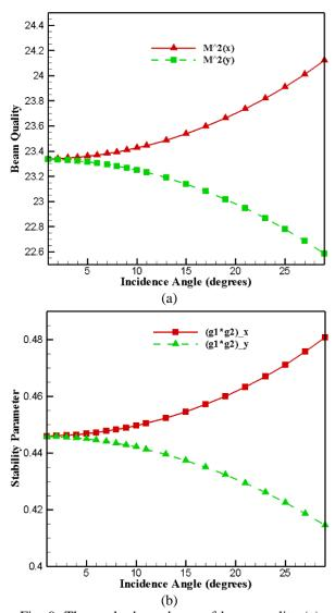
Fig. 9. The angle dependency of beam quality (a) and resonator stability (b) in V-shaped dumped cavity.
