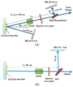
Fig. 5. Cavity-dumping resonators: (a) V-shaped and (b) L-shaped
