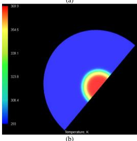
Fig. 12. (a) thermography of disk surface in maximum pump power and (b) simulation of temperature distribution of the disk surface.
