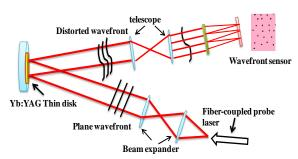
Fig. 1. Schematic of the setup used for measurement of the disk's radius of curvature.
