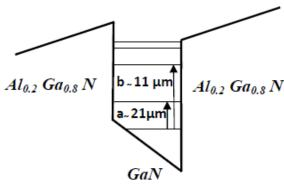
**Fig. 2** Energy diagram for the proposed structure, and the possible transitions, 'a' and 'b'.  $(l_x=l_y=9nm, and l_z=3nm)$
