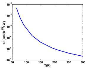
**Fig. 11** The variation of the specific detectivity as a function of temperature for GaN QDIP (lx=ly=10nm and lz=3nm) in applied bias of 0.5 V.
