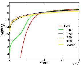
**Fig. 6** The logarithm of normalized responsivity as a function of the external electric field for the different temperatures in GaN QDIP with  $(l_x=l_v=10\text{nm} \text{ and } l_z=3\text{nm})$ .
