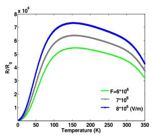
**Fig. 7** Temperature dependent of the normalized responsivity for different external electric fields in GaN QDIP with  $(l_x=l_y=10 \text{nm} \text{ and } l_z=3 \text{nm})$ .
