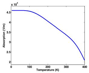
**Fig. 4** The peak of absorption coefficient for the transition 'b' vs. temperature. The GaN QD size in x-y plane and z direction is considered  $(l_x=l_v=10 \text{nm})$ , respectively.
