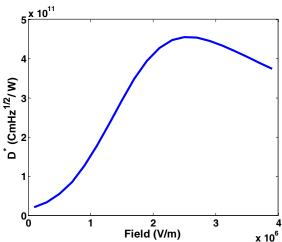
**Fig. 10** The variation of the specific detectivity for GaN QDIP (lx=ly=10nm and lz=3nm) with external electric field in T=66 K.
