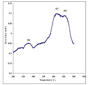
**Fig. 1** DTA curve of 41.5P<sub>2</sub>O<sub>5</sub>, 21Na<sub>2</sub>HPO<sub>4</sub>, 21PbF<sub>2</sub> - 16NaF - 0.5Eu<sub>2</sub>O<sub>3</sub> glass.
