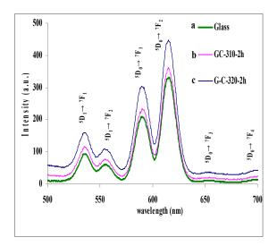
**Fig. 5** Down conversion emission spectra of Eu<sup>3+</sup> doped (a) Glass, (b) GC-310-2h, and (c) GC-320-2h samples (excited at 392 nm).
