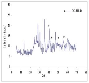
**Fig. 2** (a) XRD patterns of GC-310-2h sample with  $PbF_2$  phase (#).
