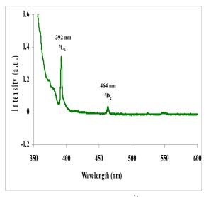
Fig. 3 Absorption spectrum of Eu<sup>3+</sup>: Glass sample.
