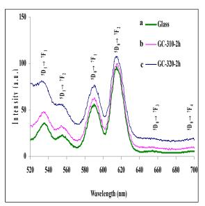
**Fig. 6** Down conversion emission spectra of Eu<sup>3+</sup> doped (a) Glass, (b) GC-310-2h, and (c) GC-320-2h samples (excited at 464 nm).
