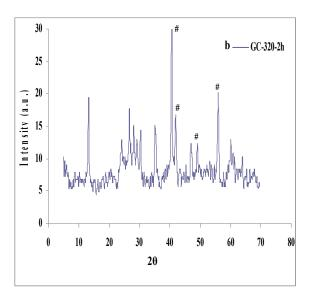
**Fig. 2** (b) XRD patterns of GC-320-2h with PbF<sub>2</sub> (#) dominated phase.
