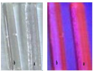
**Fig. 8** Transparent Eu<sup>3+</sup> doped glass (a) and glass ceramic (b) at ordinary light (left), under UV lamp (right).
