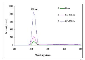
**Fig. 9** Upconversion emission spectra of Eu<sup>3+</sup> doped (a) Glass, (b) GC-310-2h, and (c) GC-320-2h samples (excited at 710nm).
