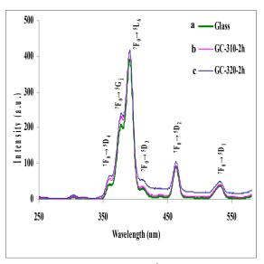
**Fig. 4** Excitation spectra of Eu<sup>3+</sup>doped (a) Glass (b) GC-310-2h and (c) GC-320-2h samples (monitored at 612 nm).
