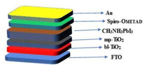
Fig. 1. Schematic illustration of structure of perovskite solar cell: FTO/bl-TiO<sub>2</sub>/mp-TiO<sub>2</sub>/Perovskite (CH<sub>3</sub>NH<sub>3</sub>PbI<sub>3</sub>)/ Spiro-OMETAD /Au.
