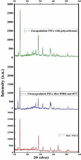
Fig. 7. XRD patterns of the encapsulated, unencapsulated and reference perovskite solar cell.
