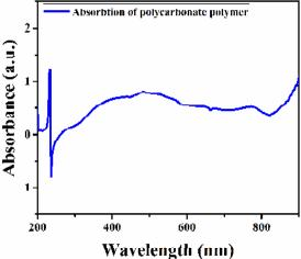
Fig. 3. UV-vis absorption spectrum of the polycarbonate.
