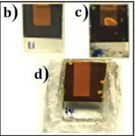
Fig. 5. (a) Schematic view of the structure of a perovskite solar cell encapsulated with polycarbonate and glass polymer and sealed with UV adhesive, (b) capsule-free reference structure, (c) cell encapsulated with clear polycarbonate polymer without glass coating, and (d) final capsule structure with polymer, glass coating, and sealing with adhesive, which after exposure to moisture and heat, keeps a percentage of its stability.
