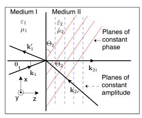
**Fig. 1** (Color online) Refraction into a lossy DNG material. The planes of constant phase are perpendicular to the propagation direction and make a negative angle  $\theta_2$  with the interface, but the planes of constant amplitude are parallel to the interface.
