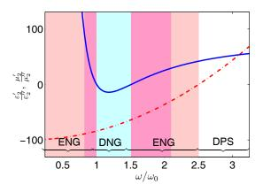
**Fig. 5** (Color online) The plot of  $\varepsilon_2'/\varepsilon_2''$  and  $\mu_2'/\mu_2''$  as a function of normalized frequency  $\omega/\omega_0$  for a lossy metamaterial described by Eqs. (17) and (18) with and  $\omega_{ep} = 10 GHz$ ,  $\omega_0 = 4 GHz$ , F = 0.56 and  $\gamma_e = \gamma_m = 0.01 \omega$
