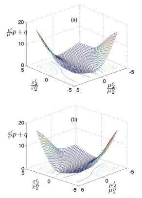
**Fig. 4** The quantity  $\frac{\alpha'}{\alpha''}p+q$  as functions of  $\varepsilon'_2/\varepsilon''_2$  and  $\mu'_2/\mu''_2$  for (a) TE and (b) TM polarizations, respectively.
