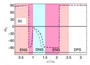
**Fig. 6** (Color online) a) real refractive index  $N_2$  and b) real refractive angle  $\theta_2$  as functions of normalized frequency  $\omega/\omega_0$  for three different incidence angles  $\theta_1=0^\circ$  (solid lines),  $\theta_1=30^\circ$  (dash lines) and  $\theta_1=60^\circ$  (dash-dot lines). Other parameters are the same as Fig. 5.
