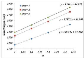
Fig. 4. The wavelength of LSPR peaks Vs. the refractive index of the surrounding medium for THS with different number of steps from 1 to 3. Structure radius=5nm is fixed.
