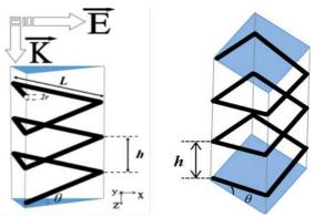
Fig. 1. Schematic model and geometric parameters of the square and triangular chiral plasmon nanosensors.
