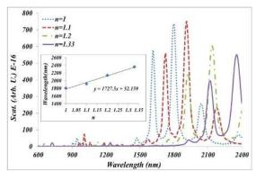
Fig. 7. Scattering cross-sections of SHS with number of steps=3 and structure radius *r*=5nm under normal incidence light for various refractive index from 1 to 1.33. Inset: The wavelength of LSPR peaks Vs. the refractive index of the surrounding medium.
