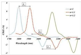
Fig. 8. CD spectra of the SHS with number of steps = 3 and structure radius r=5nm Vs. wavelength for the different refractive index of the surrounding medium.
