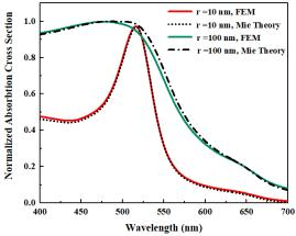
Fig. 1. Comparing the results obtained using simulation by FEM method with those calculated by using Mie theory for the small and large spherical
