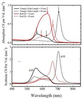
Fig. 6. Absorption (a) and Scattering (b) CS per NP volume for a rod with diameters of 12 and 36 nm and an aspect ratio (L/D) of 3, and the equilateral triangular prism with a sides of 30 and 90 nm and the height of 10nm. The values of scattering CS of triangular NP are magnified by a factor of 10 for better visibility.
