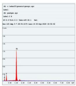
Fig. 3. EDX analysis of the Kapton substrate.
