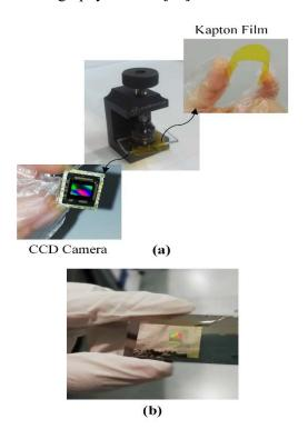
Fig. 1. (a) Sample preparation process, and (b) the fabricated plasmonic crystal.
