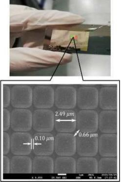
Fig. 2. SEM image of the fabricated plasmonic crystal.
