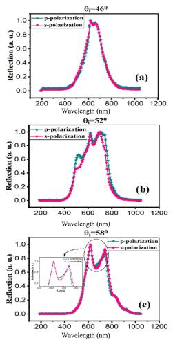
Fig. 5. Reflection spectra of the plasmonic structure under different incidence angles of (a) 46°, (b) 52°, and (c) 58° for s and p-polarization.
