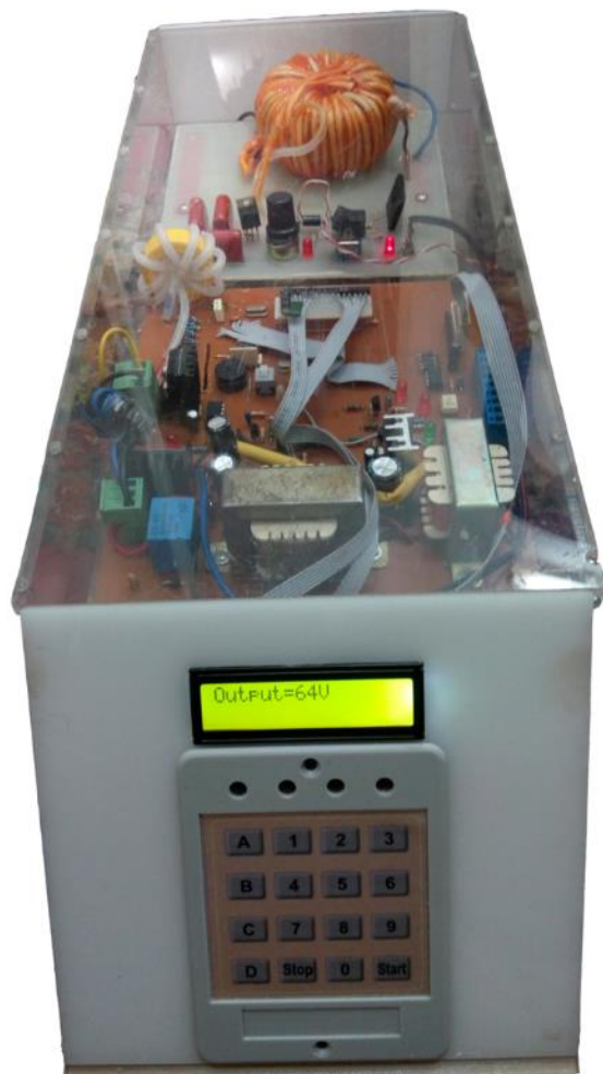
Fig. 1. A view of home-made pulsed light driver
