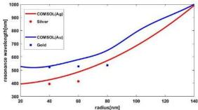
Fig. 4. Comparison of COMSOL (lines) and experimental data(dots) plasmon resonance redshift driven by gold and silver larger nanospheres.
