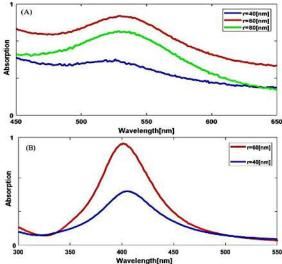
Fig. 2. Absorption spectra for (A) gold and (B) silver nanoparticles was achevied experimentally by UV-visible spectrometer.
