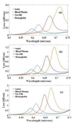
Fig. 6. The confinement loss spectra with different sensing layers and different pitch sizes  $\Lambda$ = (a) 1.9  $\mu$ m (b) 2  $\mu$ m (c) 2.1  $\mu$ m The other parameters are d = 1.4  $\mu$ m, and d<sub>Au</sub> = 45nm.
