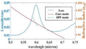
Fig. 2. The confinement loss spectra of the fundamental core mode and the dispersion relation as function of the wavelength for structure with water as a sensing layer (n=1.333). The other parameters are  $\Lambda = 1.9 \mu m$ , d = 1.4 $\mu m$ , and d<sub>Au</sub> = 45nm.
