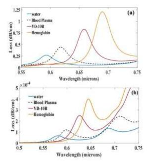
Fig. 5. The confinement loss as a function of the wavelength for different sensing layers and different hole diameters d=(a) 1.4 $\mu$ m and (b) 1.8 $\mu$ m. The other parameters are  $\Lambda=2\mu$ m, and  $d_{\rm Au}=45nm$ .
