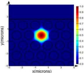
Fig. 3. Fundamental mode distribution for structure with  $\Lambda = 1.9 \mu m$ ,  $d = 1.4 \mu m$ , and  $d_{Au} = 45 nm$ .
