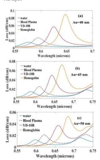
Fig. **4.** The confinement loss as function of wavelength for different sensing layers and different values of the gold layer thickness of  $d_{Au} = (a)$  40nm, (b) 45nm, and (c) 50nm. The other parameters are  $\Lambda = 2\mu m$ , and  $d = 1.6\mu m$ .
