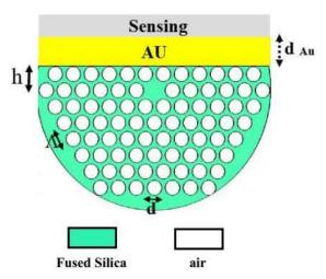
Fig. 1. proposed D-Shaped SPR based PCF biosensor.
