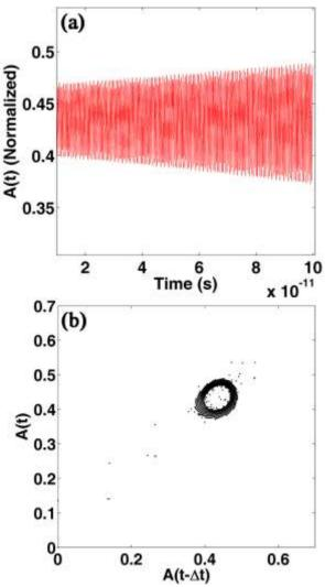
Fig. 4. (a) Time evolution and (b) phase portrait for  $E_F$ =0.49eV in arm II (case II) of Mach-Zehnder interferometer.
