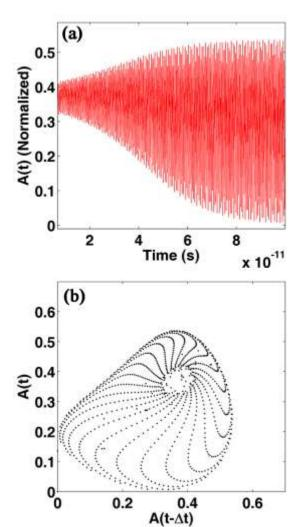
Fig. 2. (a) Time evolution and (b) phase portrait for  $E_F$ =0.4eV in arm I of Mach-Zehnder interferometer.
