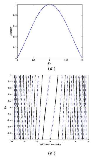
Fig. **6**. (a) The visibility of the three central diffraction fringes of a step with constant height versus the phase difference divided by  $\pi$ . (b) The plots of the locations of the intensity extremes of the step fringes versus the Fresnel variable for the phase change in the interval  $-\pi < \varphi_0 < \pi$ .
