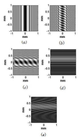
Fig. 8. The simulated fringe patterns corresponding to the wavefronts represented in Fig. 7 for the angles, (a)  $\alpha = 0$ ,  $\beta = 0$  (b)  $\alpha = 0.1^{\circ}$ ,  $\beta = 0$ , (c)  $\alpha = 0.2^{\circ}$ ,  $\beta = 0$ , n = 1.5, (d)  $\alpha = 0$ ,  $\beta = 0.6^{\circ}$ , n = 1.5, and (e)  $\alpha = 0.2^{\circ}$ ,  $\beta = 0.6^{\circ}$ , n = 1.5.
