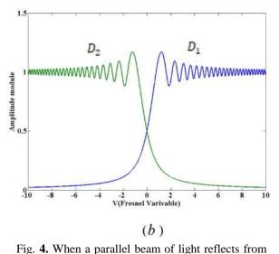
or transmits through a step of constant height, it is splitted into two parallel plane wavefronts with a common border. (a) The traces of such wavefronts on the xz plane are represented by  $\Sigma_1$  and  $\Sigma_2$ , with the common border along the y axis. (b) The moduli of the amplitudes of the diffracted wavefronts,  $D_1$  and  $D_2$ , are plotted versus distance from the common border versus the Fresnel variable.
