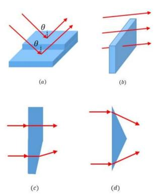
Fig. 3. Discontinuous change in the phase of a beam occurs as the beam (a) reflects from a step, or (b) passes through the neighborhood of a transparent plate edge. Discontinuous change in the phase gradient occurs as a light beam (c) passes through a transparent plate with a wedge, or (d) passes through a bi-prism.
