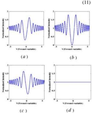
Fig. 5. The normalized intensity profiles of the fringes of the light diffracted from a step with parallel surfaces versus the Fresnel variable for  $\varphi_0 = (a) \left(m + \frac{1}{2}\right)\pi$ ,  $(b) \left(m + 1\right)\pi$ ,  $(c) \left(m + \frac{3}{2}\right)\pi$ , and  $(d) \left(m + 2\right)\pi$ , where m is an even number.
