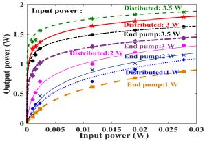
Fig. 2. Amplifier output peak power end-pumping and distributed array versus input signal power for several incident pump powers.
