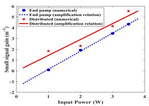
Fig. **5.** Small-signal gain of end-pumping and distributed array versus pump power at a fixed  $3.35 \times 10^{26}$  m<sup>-3</sup> concentration.
