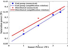
Fig. **6.** Saturation power of end-pumping and distributed array versus pump power at a fixed  $3.35 \times 10^{26}$  m<sup>-3</sup> concentration.
