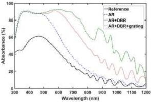
Fig. 6. The absorbance spectra of thin film Si solar cell with two coating layers of  $ZnO/TiO_2$  at four cases: 1) Reference, 2) with ARC, 3) with ARC and photonic crystal, and 4) with ARC, photonic crystal and grating, which are represented by solid, dashed, dotted and dashed-dotted lines, respectively.
