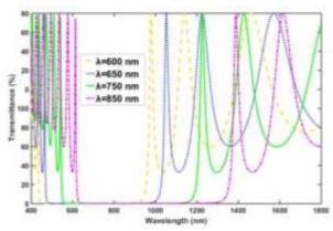
Fig. 3. The transmittance spectra of the photonic crystal at different central wavelengths.
