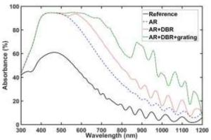
Fig. 7. The absorbance spectra of thin film Si solar cell with two coating layers of MgF<sub>2</sub>/TiO<sub>2</sub> at four cases: 1) Reference, 2) with ARC, 3) with ARC and photonic crystal, and 4) with ARC, photonic crystal and grating, which are represented by solid, dashed, dotted and dashed-dotted lines, respectively.
