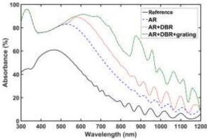
Fig. **8**. The absorbance spectra of thin film Si solar cell with two coating layers of Al<sub>2</sub>O<sub>3</sub>/TiO<sub>2</sub> at four cases: 1) Reference, 2) with ARC, 3) with ARC and photonic crystal, and 4) with ARC, photonic crystal and grating, which are represented by solid, dashed, dotted and dashed-dotted lines, respectively.
