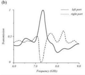
Fig. 3. (a) The electric field profile at f=7.25 GHz shows that propagation of the electromagnetic field is only allowed to the left in the waveguide. The inset shows the direction of the propagating light can change by the direction of the applied magnetic field. (b) The transmission spectrum of the waveguide shows that at f=7.25 GHz all the energy is propagated to the left port and zero energy is received at the right port.
