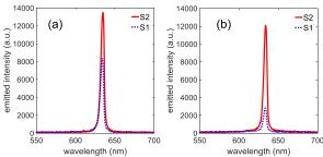
Fig. 11. Comparison between the emission spectra of the samples S1 and S2 at the excitation positions: (a) P1 and (b) P2. The pump fluence is 151.3 mJ/cm<sup>2</sup>.
