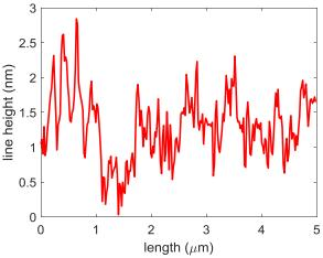
Fig. **6.** Atomic force microscope (AFM) line height plot of the glass substrate (microscope slide).
