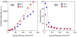
Fig. 12. Comparison between plots of: (a) maximum emitted intensity in arbitrary units, and (b) linewidth versus the pump fluence corresponding to the samples S1 and S2 at the excitation position P1.
