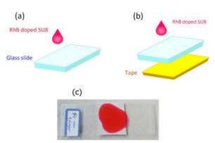
Fig. 2. Schematic illustration of the preparation method, by using drop coating technique: (a) RL sample (sample S1), (b) RL sample with a double-sided tape that is stuck to the back side of the sample (sample S2), (c) A camera photograph of the prepared sample S2.
