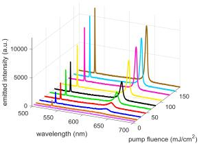
Fig. 3. Pump dependent variation of the emission spectrum corresponding to the glass substrate coated with RhB dye doped SU-8 epoxy based polymer (sample S1).
