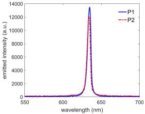
Fig. **9.** Comparison between the emission spectra of S2 (sample 2) corresponding to two different excitation positions P1 (position 1) and P2 (position 2) at the pump fluence of 151.3 mJ/cm<sup>2</sup>.
